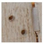
If you are mounting control horns on balsa wood surfaces, you must harden that surface to give proper support to the horns. Take a pin or Exacto knife and punch the area with a lot of holes on both sides, apply thin CA adhesive and sand smooth. Drill holes for bolts going thru the horns, put a drop of CA in the holes, redrill. This will make the area almost as hard as plywood. This procedure is not necessary if mounting horns to plywood.
