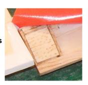
Before starting to cover aircraft, "pin the hinges". No matter what style of hinges you use, it is a good idea to pin the hinges to the airframe so they can't pull out. Drill or punch a small hole in both halves of the hinge, insert toothpick, apply a droplet of thin CA adhesive, sand smooth.
