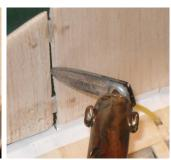
As shown in the video, do the edges and inside corners with narrow film strips. The Trim Iron works best for this. Start with the iron on low so it won't shrink the film too much. Once it is ironed on and smoothed out, turn the iron on high and
