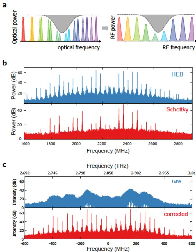
Fig. 2. (a) Schematic version of dual comb spectroscopy. Two combs with a slightly different repetition rate are detected with a square-law detector, giving rise to an RF comb that encodes the optical spectrum. (b) THz QCL dual comb spectroscopy, measured on a hot electron bolometer (HEB) and Schottky mixer [5]. (c) Computation self-correction of an unstable dual comb signal. Using this approach, even highly unstable environments can be used for dual comb spectroscopy [7].
