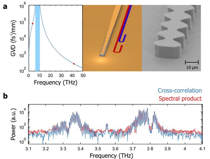
Fig. 1. (a) Dispersion engineering of a THz QCL comb. Group velocity dispersion (GVD) of GaAs at terahertz and mid-infrared frequencies (left), schematic of a double-chirped mirror that compensates dispersion (center), SEM of a double-chirped mirror (right). (b) Coherence measurement of a comb. By comparing the cross-correlation to the spectral product, first-order coherence is measured. [4], [6]
