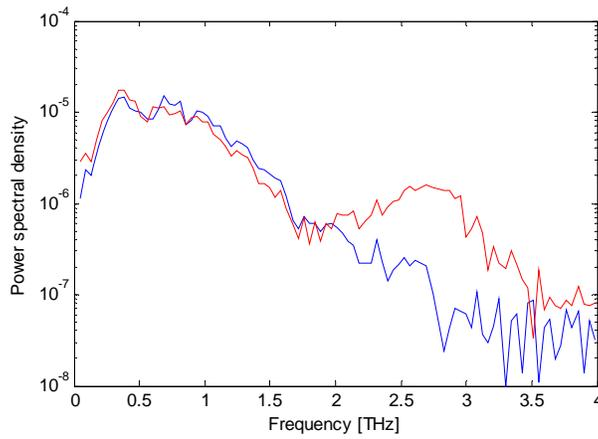
Figure 1(b): Frequency content of pulses. Two data points have been removed corresponding to atmospheric absorption lines not eliminated by purging; no additional scaling has been performed.
