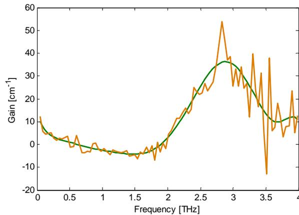
Figure 2: Gain spectra computed by dividing the logarithm of the ratio of the spectra by the device length. Green line is gain calculated from polynomial fits of data in Fig. 1(b).
