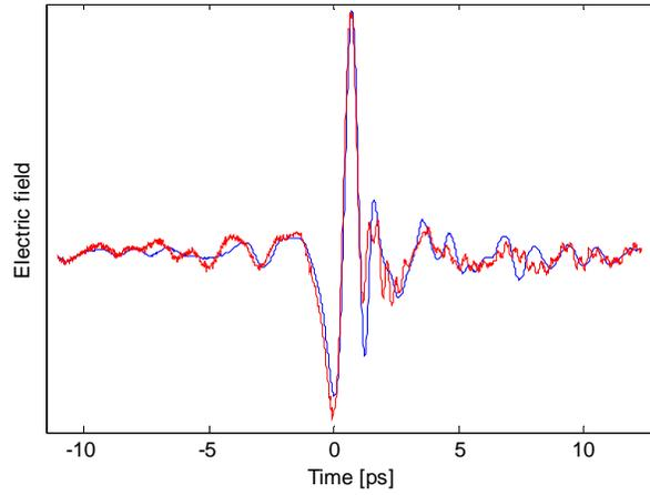
Figure 1(a): Pulse generated by device biased below threshold (5 mA, shown in blue) and above threshold (500 mA, shown in red). Gain medium is designated FL175M-M3, and has a two-well injector with a resonant-phonon depopulation scheme. Device is 80 microns wide and 1.5 mm long.
