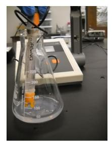
4. Gradually add the NaOH solution, with swirling, until the pink phenolphthalein color begins to persist. When near the endpoint, add the NaOH solution dropwise until one drop causes a pink color that persists for 30 seconds. If the endpoint is over-run, more acid may be added and the titration continued.
