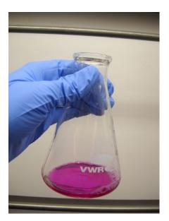
When phenolphthalein is used with The Works Toilet Bowl Cleaner, which is pale aquablue, the color changes sharply from blue to light purple. Use only 1/4 of the bottle for The Works Cleaner - it takes more NaOH to reach pH 7 than with the standard, and you may run out of solution if you use too much starting product.
