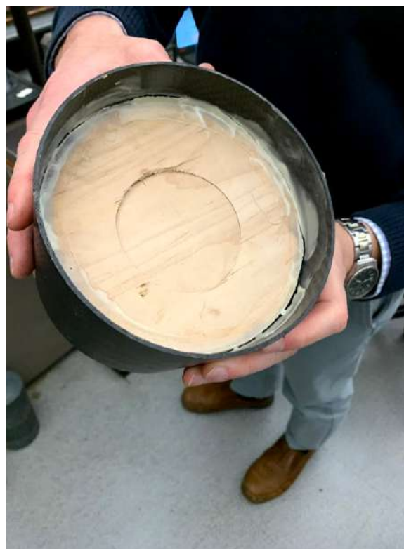
Figure 22: Plywood Failed Bulkhead
