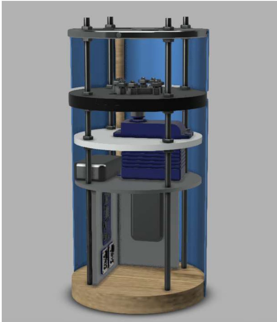
Figure 32: Model of ABS within a section of the fin can
