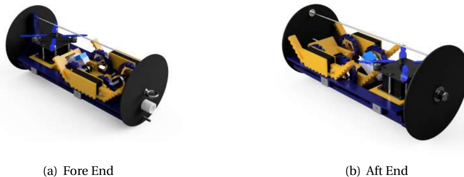
Figure 83: CAD Model of full LSRS within the Payload Bay
