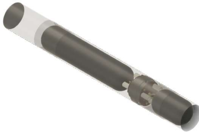
Figure 12: Assembled Recovery Body Tube
