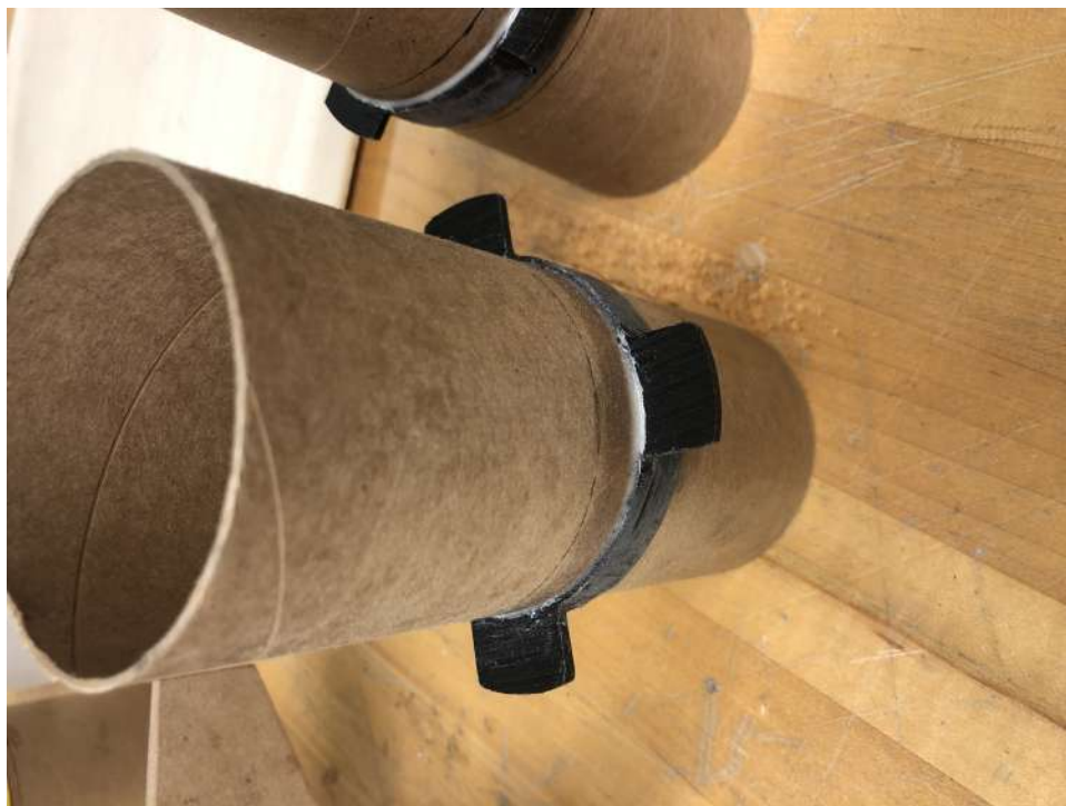
Figure 140: Sub-scale drag tabs on coupler
