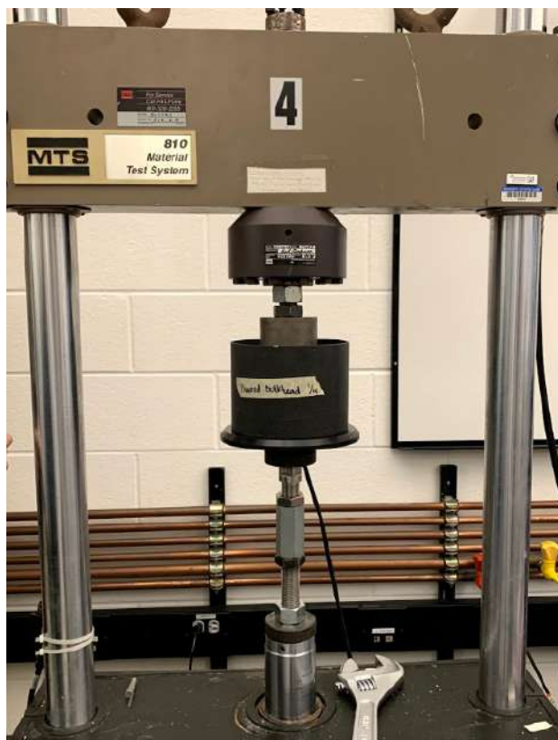
Figure 21: Load Cell Setup
