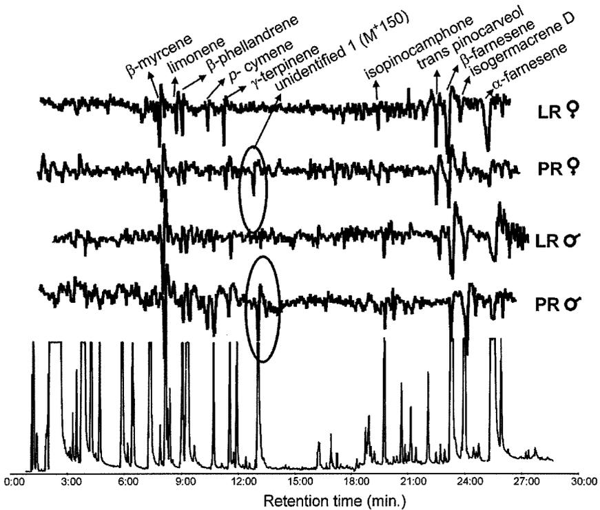
FIG. 3. Analysis of larch foliage odor as collected on a porous polymer by GC-EAD with LBM larch (LR) and cembra pine host race (PR) antennae. For further details see text and legend to Figure 1.
